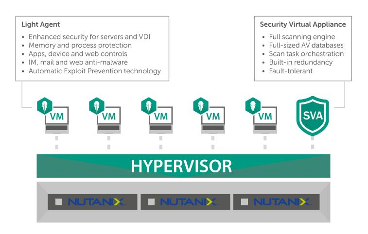
A Security Virtual Appliance (SVA) on each host scans all VMs centrally, while a powerful but lightweight agent deployed on each VM allows advanced security features, including application, device and web controls, anti-malware protection for IM, mail and web, plus advanced heuristics, to be activated.
