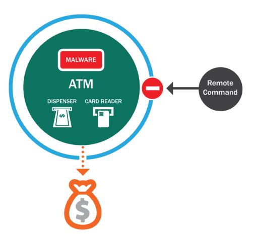
Geographically scattered ATM endpoints are ideal for the introduction of malware infections as part of a targeted attack, particularly as USB access ports and keyboards are conveniently located in a system servicing cabinet, secured only by a basic lock, at the back of the ATM itself.
